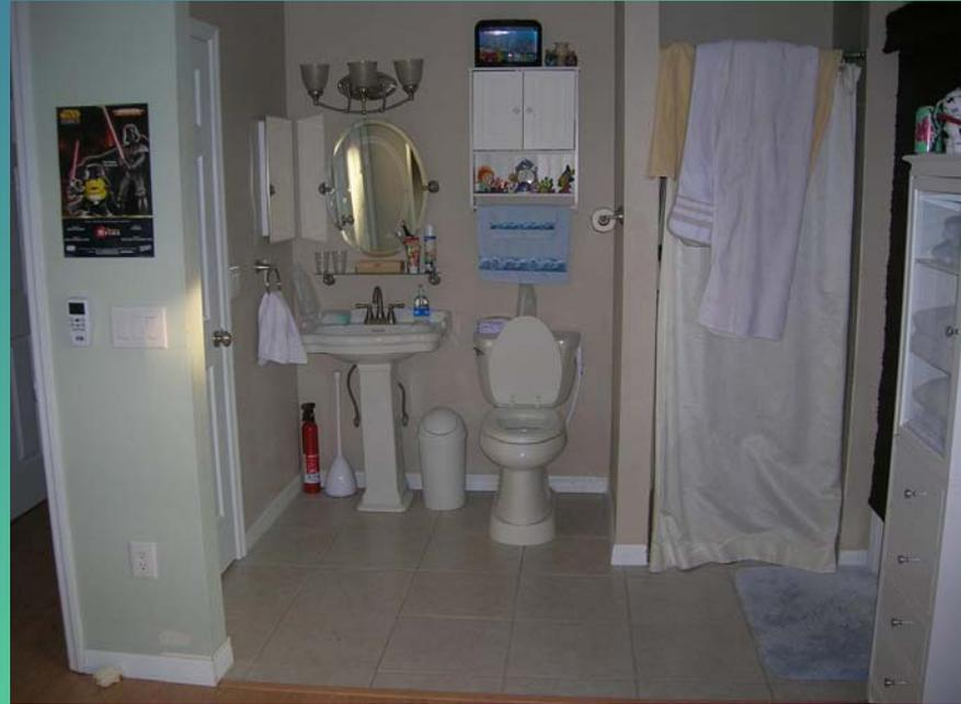
This is a picture of the pool bath it was next to the game room so we had the wall removed. This way we can roll Zachary right into his bathroom for toiletry needs. I put in a pedestal sink so he could drive up and brush his teeth at his own sink. The mirror tilts down so a person in a chair can see themselves.
